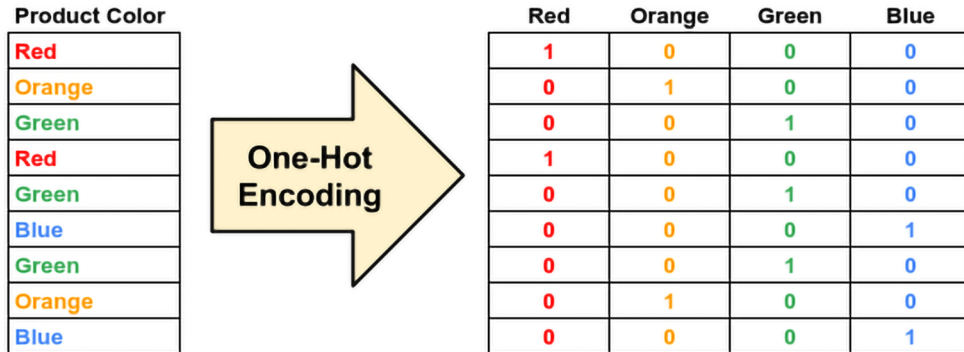
Figure 4.5 Example of one-hot encoding, 13 used for input data into neural networks in PyTorch
